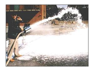
The Unifire V nozzle can be combined with a foam tube to give either low or medium expansion foam.
