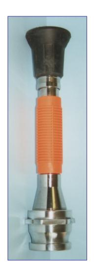
This jet/spray nozzle is operated by turning the nozzle head, producing an absolutely parallel jet with excellent range or a homogenous spray pattern. The nozzle has a baffle rod which is prismatically attached and therefore perfectly centred by water pressure, which is neutralised on all moving parts.
