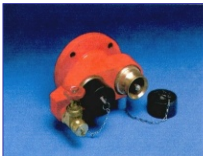
4" TWO-WAY PUMPING-IN BREECHING WITH SG IRON BODY & GUNMETAL FITTINGS
